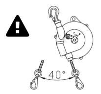
The use through overly big angles will reduce lifespan of rope. **Recommended range of** angle:  $\pm 20^{\circ}$
