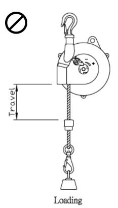
Do not twist and rub the cordage with cable during travel. Do not load over the stated capacity.
